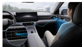
Integrated with the air conditioning outlet
